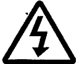
Warning, high voltage
