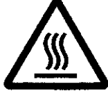
Warning, high temperature
