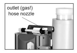
The **exhaust waste vapor condenser** enables an efficient condensation of the pumped vapors at the outlet.
