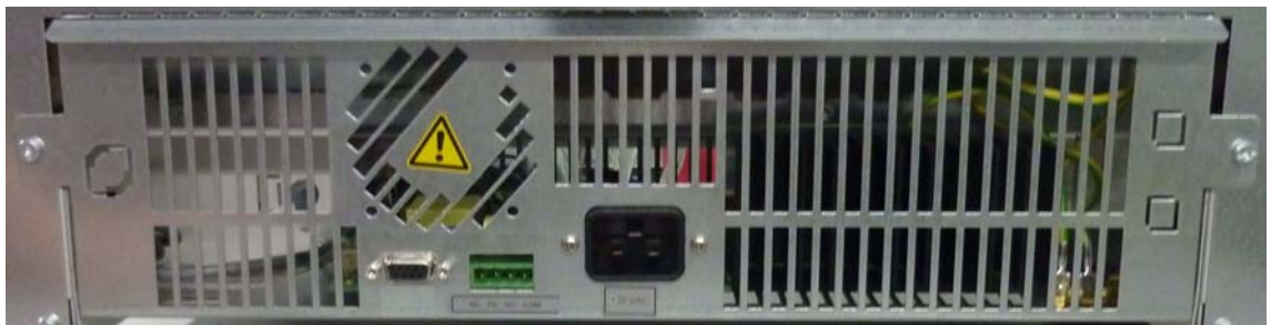
Figure 5-9 AC Power Supply Socket
