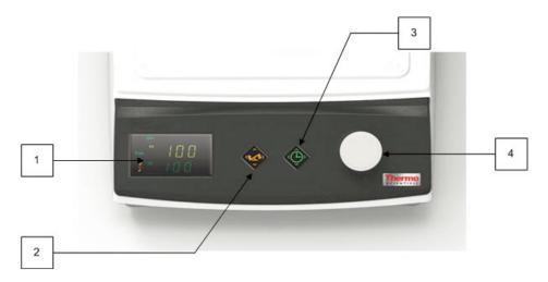
(1) VFD (Vacuum Fluorescent Display): Check status of unit on display.
