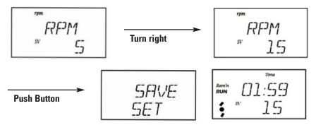
(2) Shaking stops and alarms when the time is terminated. If you press dial knob or touch button, display returns to stand by status.
