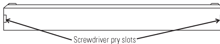
Figure 5-9. Front Cover Plate Below the Door
