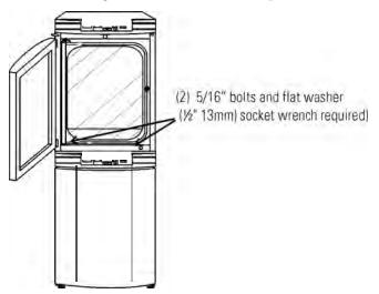
Figure 1-7. Align Slots and Bolts
