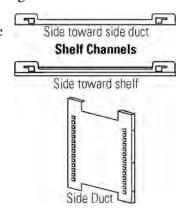
Figure 1-10. Shelf Channels and Side Duct
