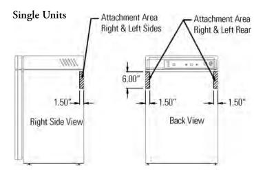
**Caution** Do not drill deeper than 1/2 inch. Exterior wrap is 18 ga. cold rolled steel. ▲
