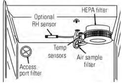
Figure 5-1. Sensor and Filter Locations
