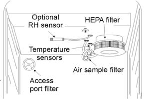
**Figure 1-9.** Filter and Sensor Locations
