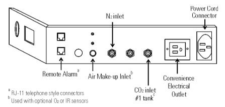
Figure 1-13. Back Panel and All Connections
