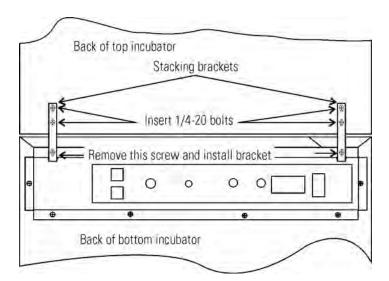
**Figure 1-8.** Two Screws From Control Panel Back
