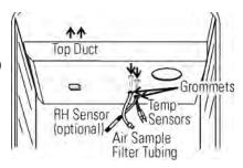
Figure 5-3. Feed Through Holes
