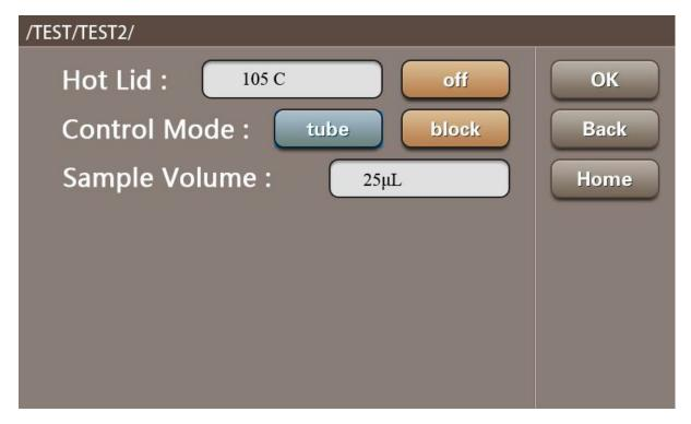
**Heated lid:** Open by default, and the default temperature is 105 °C. If needed, you also can set the temperature of the heated lid.
