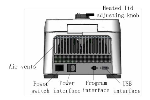
**Heated lid adjusting knob:** Adjust the height of heated lid to accommodate different reaction tubes.
