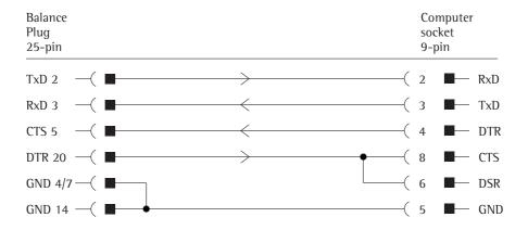
Cable type: AWG 2 specification
