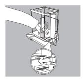
Secure the draft shield by pressing lightly on the draft shield base and moving the sliding lock device to the left
