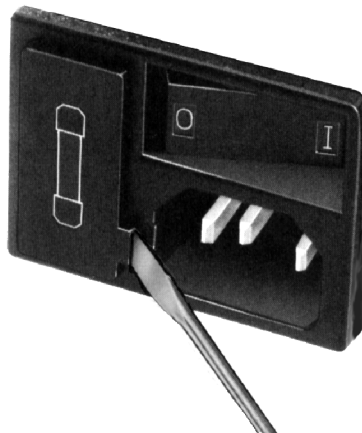
Figure 5.1: Prying open the fuse box cover.
