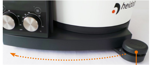
Hand lift lever: upper lift position
