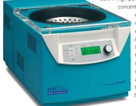
concentration chamber with electro-magnetic drive for quiet, maintenance free operation, and a fixed angle aluminium rotor for 1.5 ml microcentrifuge tubes. Simply position the system on the bench, connect the power lead and exhaust tube and look forward to faster, trouble free concentration!
