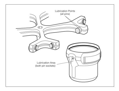
Figure 13. Lubricating Pivot Pin/Bucket Contact Areas
