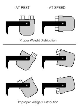
Figure 6. Examples of the Effects on the Horizontal Swing of Buckets Caused by Proper and Improper Weight Distribution
