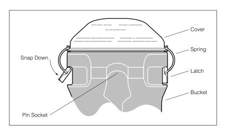
Figure 11. Securing Bucket Cover Latches
