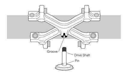
Figure 2. Rotor Yoke and Centrifuge Drive Shaft. Be sure the pin in the drive shaft is in the groove in the rotor yoke.
