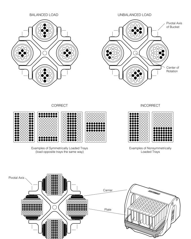
Figure 4. Examples of Correctly and Incorrectly Loaded Buckets and Carriers. Contents of opposing buckets must be the same and each bucket must be balanced on its pivotal axis.
