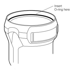
Figure 10. Proper Placement of O-Ring
