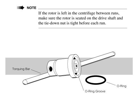
Figure 3. Rotor Tie-Down Nut and O-Ring
