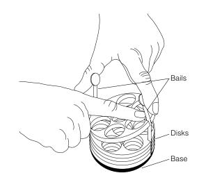
Figure 7. Assembling a Modular Disk Adapter
