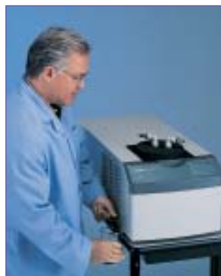
CentriVap Cold Trap collects evaporated liquid, protecting the vacuum pump.
