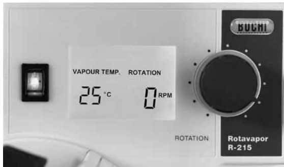
Fig. 4.8: Vapor temperature display at the R-215
