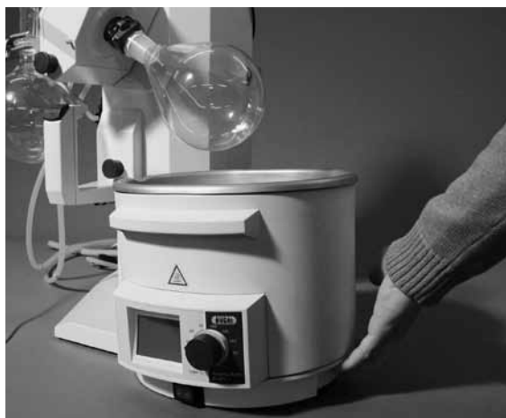
Fig. 5.1: Moving the heating bath
