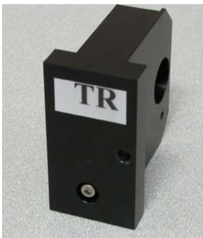
Figure 15: The “TR” cartridge, for time-resolved fluorescence assays
