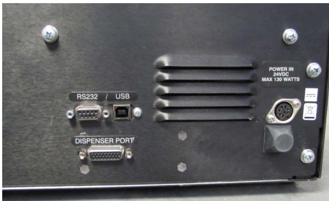
Figure 8: RS-232 serial and USB ports on the rear panel (injector model shown)
