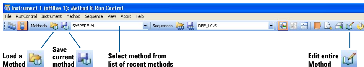
Figure 20 When you click the icon for the Single Sample Toolset , you access tools to work with methods.
