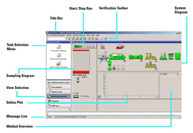
The Verification (OQ/PV) view allows an Agilent service engineer to test whether your analytical instruments and the ChemStation software are operating correctly according to predefined performance criteria.
