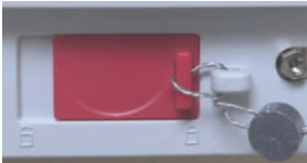
Locked with Wire Seal
