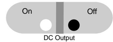
**NOTE:** The power supply output may be adjusted while operating. If you turn any of the three adjustment knobs while the D.C. Output On light is illuminated, the power supply will automatically switch to the Set Display Mode. Each display will show the set operating limit while in this mode and new limits may be set. One second after releasing the adjustment knob the power supply will revert to the Display Actual Mode.
