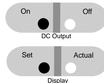
3. Gently press the Set Display key (19). The actual switch itself is located in the grey area located immediately below the word "Set" in the Set Display key. When pressed, there will be a tactile sensation, the power supply will beep and the Yellow Set Display (18) light will be illuminated. Each key on
