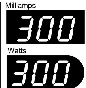
6. Gently press the D.C. Output On key (24). The Red D.C. Output On light (23) should illuminate and the D.C. output as indicated by the three displays (3, 5, 7) should rapidly increase until the operating voltage limit is reached. At this point the Yellow At Limit light (volts) (2) should be the only "at limit" light illuminated.
