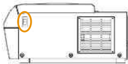
Power supply switch on the right side of the Sorvall ST 8R
