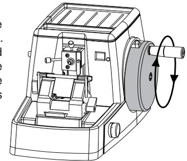
The specimen is retracted from the knife edge during the return stroke to prevent the specimen brushing against the back of the knife blade.
