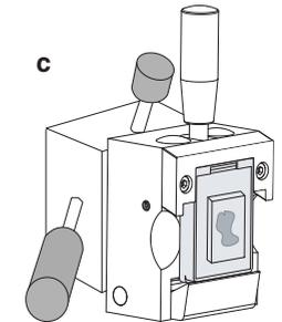
Lock the orientation head in position when the optimum orientation is obtained (d).
