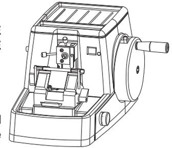
Clean the instrument regularly as part of your normal housekeeping routine, paying particular attention to the removal of wax from the area around the Knife Holder. Always remove the knife or blade, apply the handwheel brake, and lock the Knife Holder on its dovetail slide before starting any maintenance.
