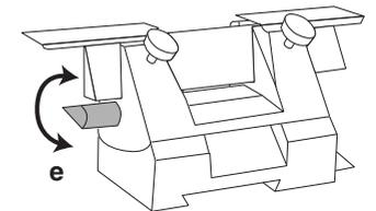
Tilt the Knife Holder with respect to the Base until the 20 graduation line aligns with the reference marker on the scale at the right hand side of the Knife Holder (*f*). This is an approximate 20° angle suitable for a new 'C' profile steel blade.
