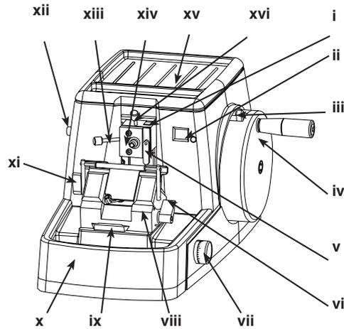
The microtome is designed for general laboratory use and features the unique 'Accu-Feed' system of precision advancement of the specimen without the need for adjustment.
