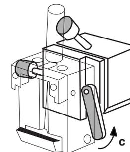
Push the Tilt Clamp lever downward to lock the assembly in its correct position.
