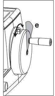
Continue turning the handwheel and advancing the specimen until clean sections of the specimen are taken. Apply the handwheel brake when trimming is completed and the specimen presents a clean smooth surface to the knife.
