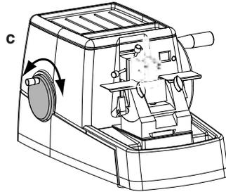
Silence the alarm when the end of travel limit is reached by moving the specimen head to within the normal operating range. Use the Coarse Advance Knob (*c*) to do this.
