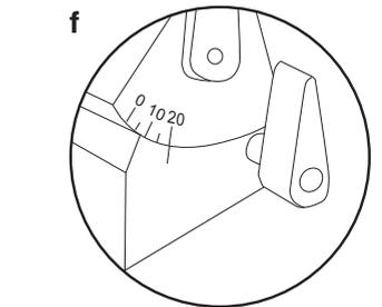
Lock the Knife Holder at the set angle by pushing the Knife Angle Lock Lever away from you.
