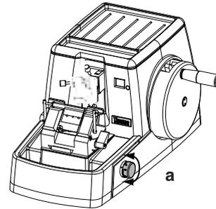
Release the handwheel brake and turn the handwheel clockwise until the handle of the handwheel is in the 2 o'clock position, and the specimen is just about to be cut.
