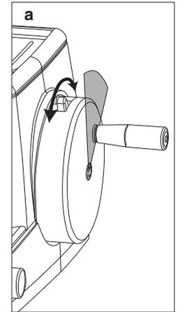
On the Cassette Clamp pull the quick release lever forward, insert the cassette, and release the lever (b). Check that the cassette is clamped firmly.
