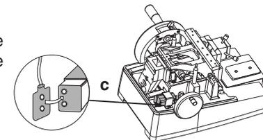
Return the outer cover to an upright position at the front of the microtome and re-make the electrical connections to the printed circuit board.
