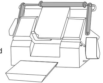
The Knife Guards of the Universal Knife Holder comprise two platforms - one either side of the cutting aperture. They require no adjustment or setting up.
