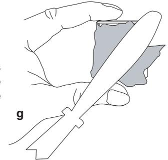
Use a scraper, plastic spatula or ParaTrimmer to remove excess wax from the sides, ends, and back of the cassette (*g*). The cassette must be able to mount squarely on the Specimen Clamp.
