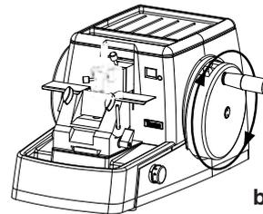
One complete revolution of the handwheel is required for each section (b). Sectioning is best performed by turning the handwheel clockwise slowly and at an even speed from the 2 o'clock position and round to 2 o'clock again. Turning the handwheel at too high a speed can compress the specimen, and cause poor ribbon adhesion.
