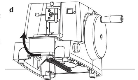
Remove the Top Tray from the instrument (*e*). Access to the transit fixings is via the outer cover of the instrument. This cover is retained by two spring clips that connect with shaped pillars mounted on the main frame inside.
