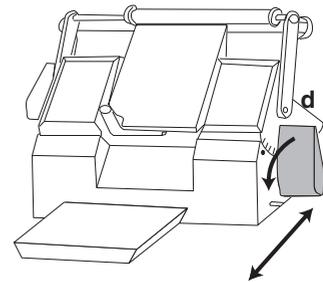
During normal operation the specimen advances by the distance set by the Section Thickness Control (*b*) as each successive section is cut. The maximum travel available is 16mm. During the course of specimen travel the indicator shows red with green when travel is available in both directions.
