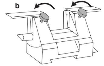
Slide the knife into position under the Knife Clamps (*c*), then tighten both Knife Clamp Screws by turning them clockwise .
