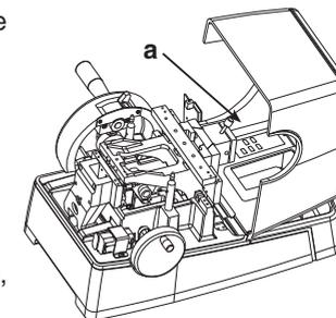
**DO NOT DISCARD THE TRANSIT FIXINGS. RETAIN THEM IN A SEALABLE POLYTHENE BAG FOR FUTURE USE. (NOTE THAT THE SCREWS CAN BE REFITTED AND KEPT IN SITU IF REQUIRED - MAKE SURE THAT THEY ARE SECURELY SCREWED INTO PLACE)**
