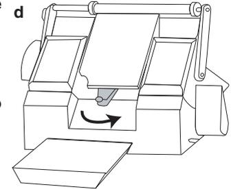
Push the Blade Clamp to the right (anti-clockwise) to lock the blade firmly in its cutting position (d).
