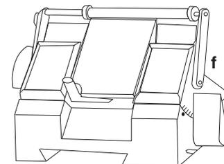
The **0322 Disposable Blade Holder** is designed for use with High profile disposable blades.
