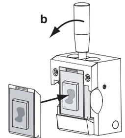
Use the vertical and horizontal tilt controls as appropriate to orientate the specimen correctly with respect to the knife edge (c).
