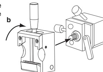
Loosen the Tilt Clamp lever (c) by moving it upward, then align the Specimen Clamp to suit. You can rotate the Specimen Clamp through 360° to obtain the best setting. Use the Vertical and Horizontal tilt knobs to adjust the orientation of the Specimen Clamp.
