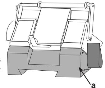
The Finesse 325 microtome has the Coarse advance knob fitted towards the back of the left hand side panel of the instrument. The Coarse Advance knob turns clockwise for specimen advancement.
