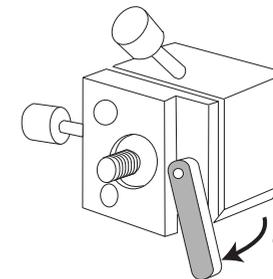
Fit the Specimen Clamp on the threaded bolt at the end of the Orientation Head, then screw it clockwise to tighten it in position (b).
