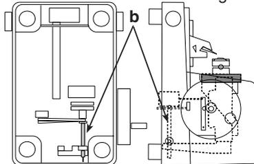
Loosen the two Knife Clamp Screws at the front of the Solid Knife Holder by turning them anti-clockwise (*b*).
