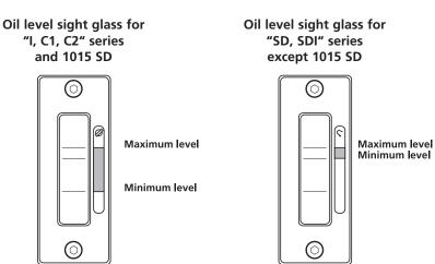
**Note:** Optimum pump performance and service life are obtained when the oil level is between the maximum level and the minimum level.
