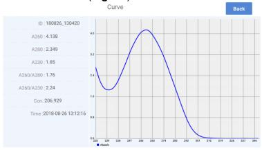
Fig. 15 Nucleic Acid Sample Absorbance Curve (220 – 350nm).
