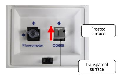
Fig. 7 OD600 & Fluorometer Port
