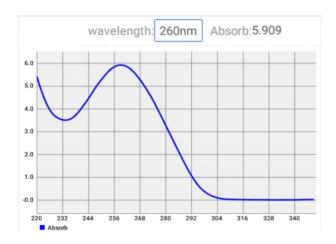
Fig. 13 Nucleic Acid Sample Absorbance Curve (220nm – 350nm)
