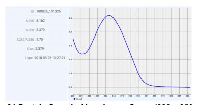
Fig. 21 Protein Sample Absorbance Curve (220 - 350nm)
