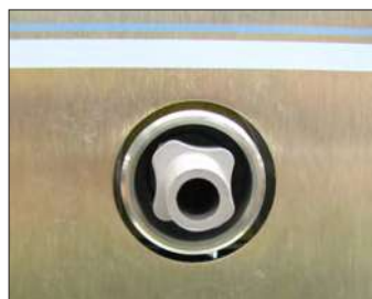
Installed Drain Fitting with Cap Removed
