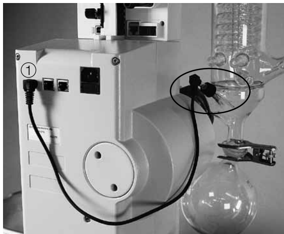
Fig. 5.14: Vapor temperature sensor
