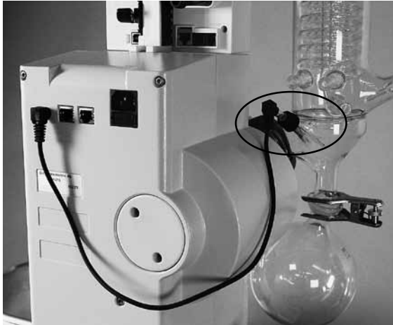
Fig. 4.7: Vapor temperature sensor
