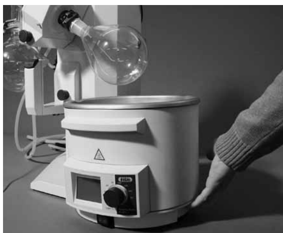
Fig. 5.1: Moving the heating bath
