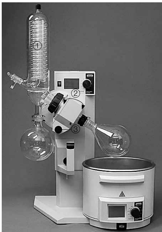
Fig. 6.3: Immersion angle of the evaporating flask into the heating bath
