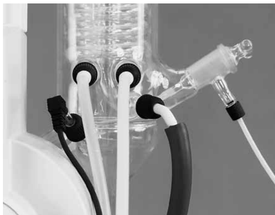
Fig. 5.9: Cooling water tubes
