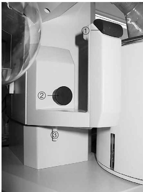
Fig. 6.4: Lowering and raising the evaporating flask
