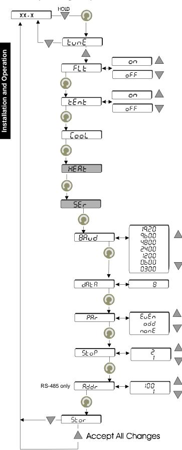
The Setup/Tuning Loop is used to configure the controller temperature display and various operating parameters. To enter the loop you must be displaying the reservoir fluid temperature and
