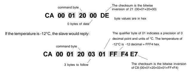
The master sets parameters in the chiller by sending one of the Set Functions as shown in Table 1. The master does not send a qualifier byte in the data field. The master should be preprogrammed to send the correct precision and units (it could also read the parameter of interest first to decode the correct precision and units needed).
