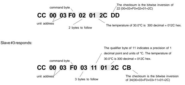
For example, if the master wants to set the setpoint to 30°C for unit #3, it would send :
