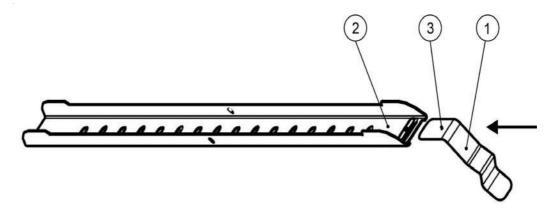
Figure 5-1 Sliding the Retaining Spring into the Support Rail
