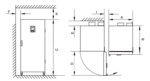
Figure 3-2 Floor Stand Incubators, dimensions and required clearances
