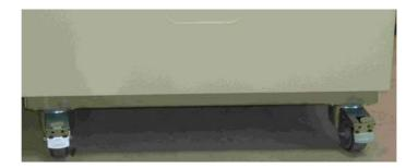
The floor stand units come equipped with four (4) casters. The lever for releasing the caster is located above the locking lever. After positioning the unit in its installation location ensure that the locking levers are pressed down on the casters.
