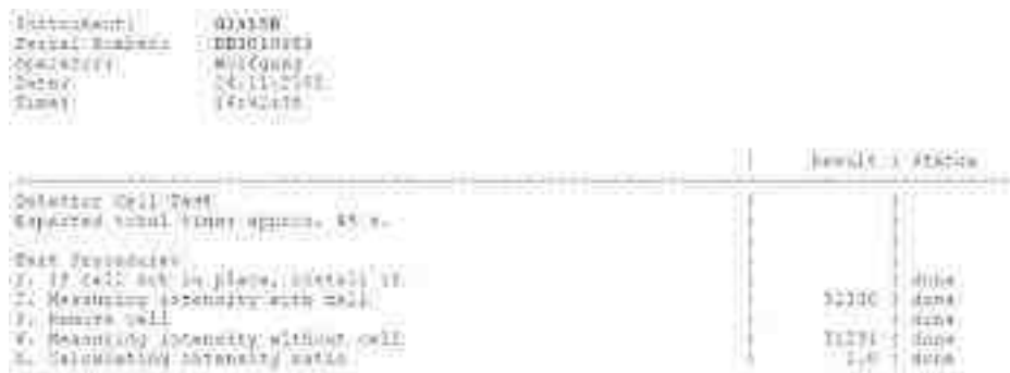
Figure 45 Cell Test Results (report) with no flow cell inserted
