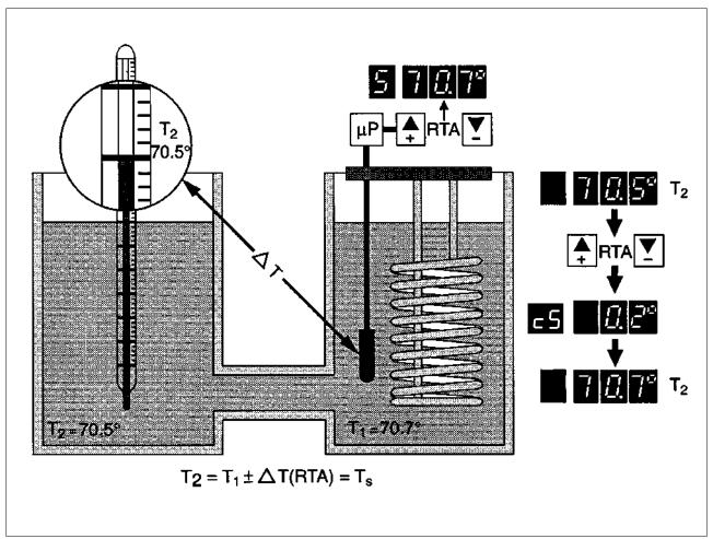
Set value programmed at the circulator  $T_{set} = 70.7^{\circ}C$
