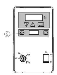
Quite often closed external systems cannot be prefilled as suggested. In this case the internal bath of the unit has to be filled to the max. level. After starting the unit, the pump will feed the necessary liquid to the external system. Should the demand be higher than the volume difference between high and low, the low liquid level sensor will be activated and the pump switched off.
