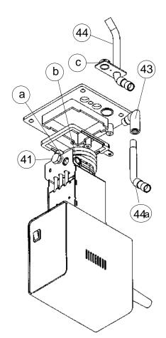
Mount the temperature control module with plate to the bath bridge.
