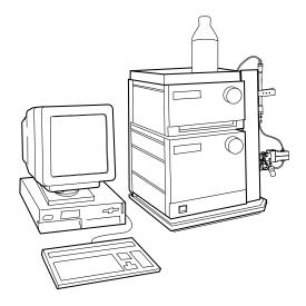
In its standard configuration, ÄKTAFPLC consists of a compact separation unit including modules and components, and a personal computer running UNICORN™ software version 4.12 or higher to control the separation unit. A fraction collector, Frac-900 or Frac-950, is also included. A hinged rack allows easy attachment of optional equipment when expanding the standard configuration.
