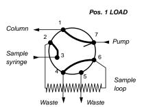
Note: If the syringe is taken out before the sample is injected onto the column, self-drainage can occur and the loop will be emptied.
