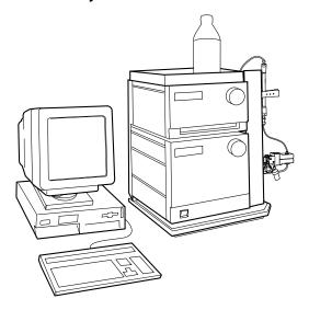
ÄKTAFPLC consists of a compact separation unit comprising modules and components, and a personal computer running UNICORN software version 4.12 or higher to control the separation unit. A fraction collector is included in the standard configuration.
