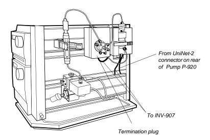
The UniNet-2 data communication chain, which controls the valve(s) and the mixer comes from the rear of Pump P-920. The chain is terminated at the injection valve with a termination plug.
