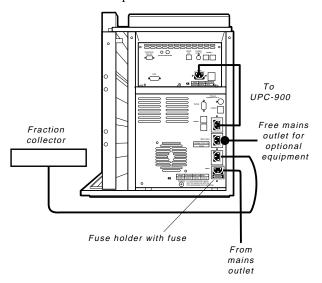
To open the fuse holder, remove the mains inlet cable to the system. Use a small-bladed screwdriver to lever the holder outwards.
