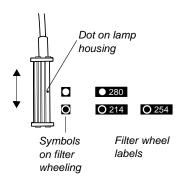
Note: The new wavelength is not automatically registered in UNICORN. This must be entered by the user. When starting a method, a question appears in which the user is prompted to state the wavelength to be used in the run.
