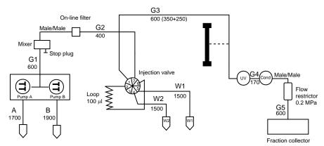
The G3 capillary is mounted at the factory as a column bypass. It is initially used during the installation test. When the test is complete and a column is to be fitted, the G3 capillary can be cut and used to connect the column. The figures state the length in millimetres of the prefabricated capillaries.
