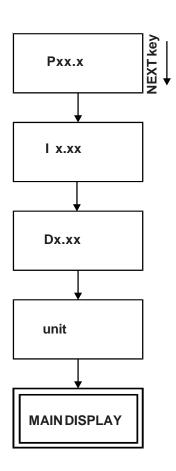
The setup loop is used to adjust the PID control and change the temperature scale. (Preset PID values are P = 1.2, I = 0.20, D = 0.00.) To enter the setup loop, from the temperature display press and hold**NEXT** for three seconds. The display will indicate **Pxx.x. NOTE:** If a key is not depressed within 60 seconds, a "time out" will occur and the display will revert to the fluid temperature.
