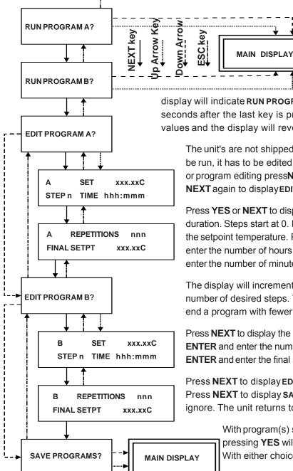
The controller can store up to two programs, each with as many as ten steps. (Refer to the Setup Loop on the next page for other options.) A sample program is shown on page 21
