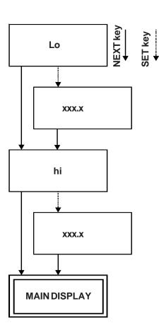
To enter the calibration loop, from the main display press and hold the up arrow key while pressing**ENTER - NEXT - ENTER**. The display will indicate **Lo** (low calibration temperature).
