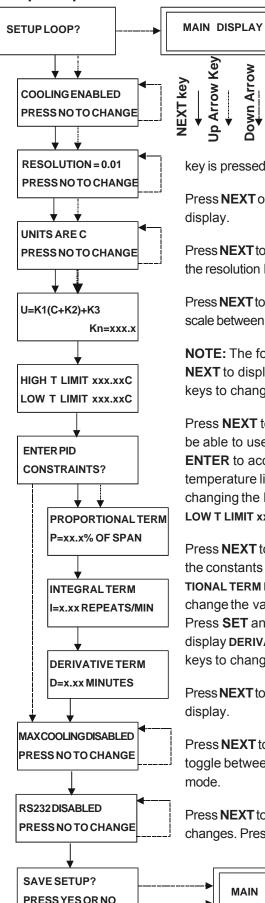
The setup loop is used to change the display resolution, change the temperature scale, change temperature limits, adjust the PID values, and enable/disable RS232 communications.
