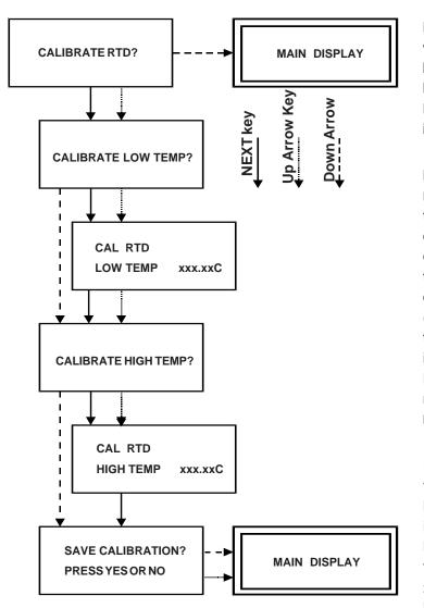
Run the temperature to a suitable low-end value. Once stabilized enter the calibration loop. From the main display press and hold **NEXT** while pressing, within three seconds, **ENTER - NO - ENTER**. The display will indicate **CALIBRATERTD**?
