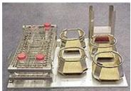
Custom spring racks (photo on Left) allow for a combination of large flasks, microtiter plates and tubes on a given platform.
