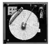
The chart recorder has a back-up battery system enabling a period of continuous operation if power is lost. Battery life varies by manufacturer as well as voltage level remaining. If full batter power is available, back-up power for the temperature chart recorder is available for up to 14 hours.
