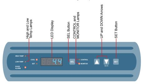
Horizon Series™ temperature monitor and control interface
